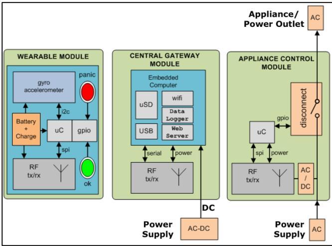
Fig. 2. Detailed architecture of iSeiz sub-systems.
