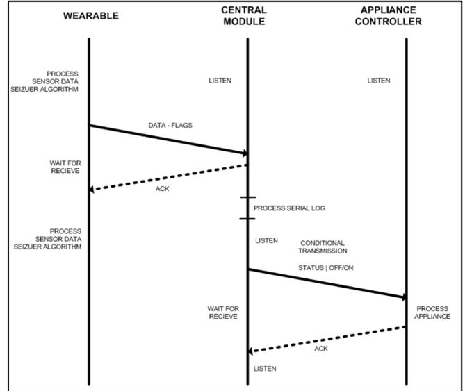
Fig. 3. The timing diagram of the signals exchanged between the three modules.
