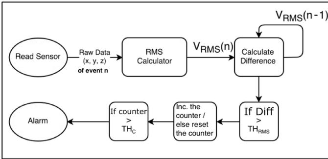
Fig. 5. Details of seizure detection algorithm.
