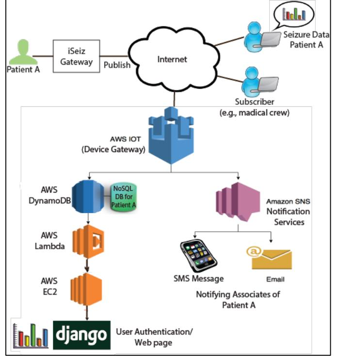
Fig. 4. AWS cloud architecture of the iSeiz system.
