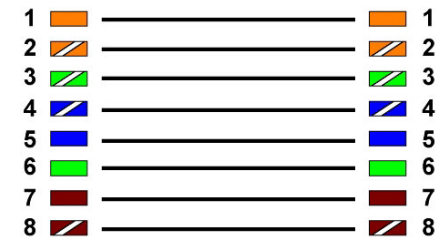
EIA/TIA T568B Straight Through Diagram
