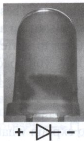
Figure 20. The positive and negative sides of a LED.
