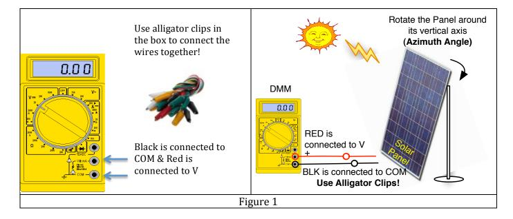
2- Rotate the panel around its vertical axis until you get the maximum voltage reading from the digital multi-meter (DMM). This is called changing the solar **azimuth angle** (see Figure 1). Secure the solar panel.
