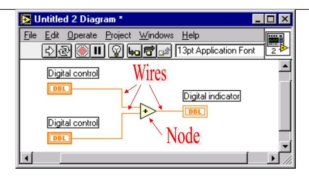
A LabVIEW VI is held together by <u>wires</u> connecting nodes and terminals; they deliver data from one source terminal to one or more destination terminals.
