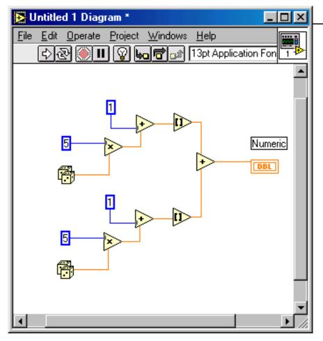
This wiring diagram simulates the rolling of 2 dice and their addition to form a number from 2 through 12.
