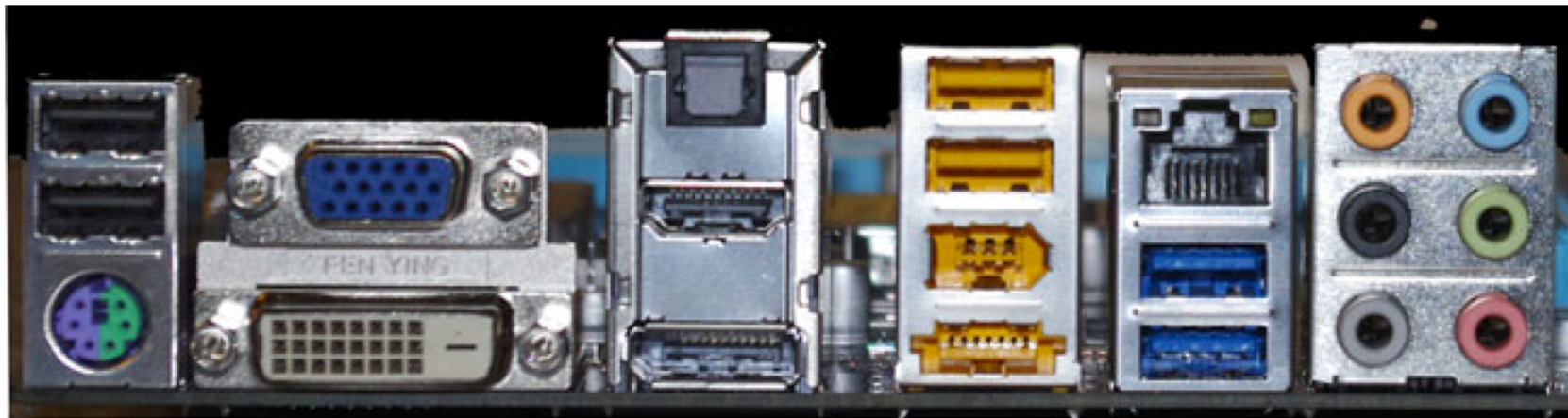
USB 2.0 USB 2.0 PS/2 VGA DVI Optical S/PDIF HDMI DisplayPort USB 2.0 USB 2.0 1394a eSATA RJ45 USB 3.0 USB 3.0 Audio Jacks Sub Line In Rear Out Side Mic In
