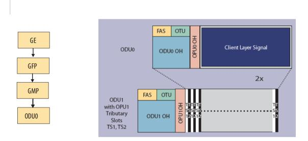
Figure 9: 1 GigE and ODU0 mapping
