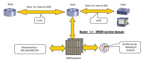
Figure 2: High-speed Ethernet applications
