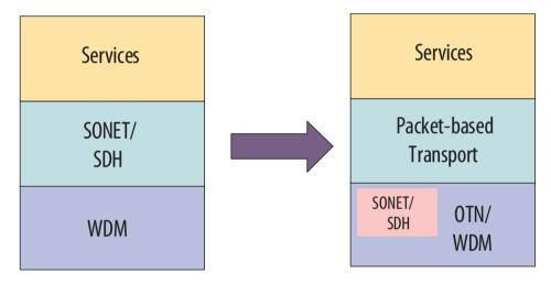
Figure 4: Migration to packet and optical transport networks
