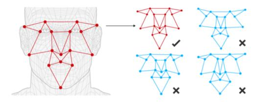
Facial recognition software reads the geometry of a face captured from a photo or video to create a unique code or 'faceprint'
